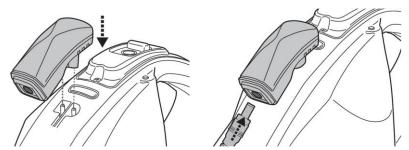
3. Connect the external adaptor to the power source. Once the robot begins charging, the indicator light on the external adaptor will turn red.
