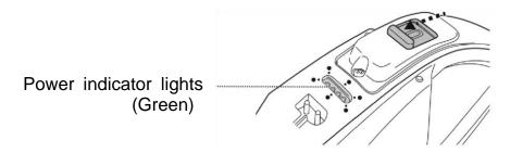
3. Immerse the robot into the water and operation will automatically begin as water level covers the sensors at the top of the swivel head. Let the robot sink to the pool floor and observe the cleaner's first forward and reversed movements across the pool bottom. If the robot runs along the pool wall instead of perpendicular to it, reposition it to make sure that its front/back faces the pool wall.
